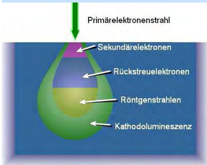
By interaction of the energetic primary electron beam with the sample, Secondary *Electrons* (SE), *Backscatter Electrons* (BE), Auger *Electrons* (AE), X-rays and, under some conditions, light photons (*Cathodo-Luminescence* CL) are released.
